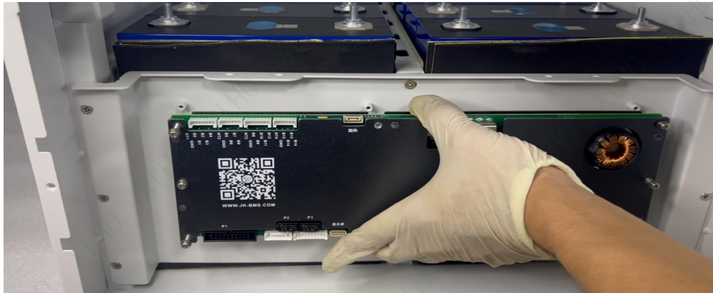
Step 4:Mount the BMS on the front panel(B-icon needs to be facing up)
