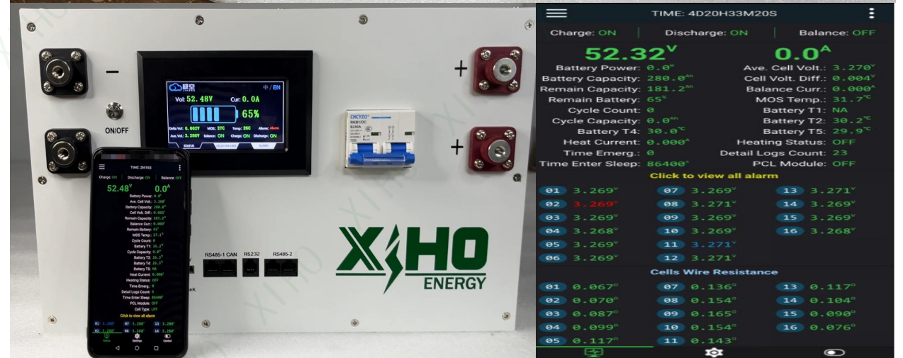
Step12:Close the cover panel, secure the screws, power on the device, and connect to your smartphone via Bluetooth to view battery pack information
