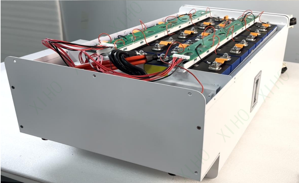
Step11:Close the front panel and secure the screws
