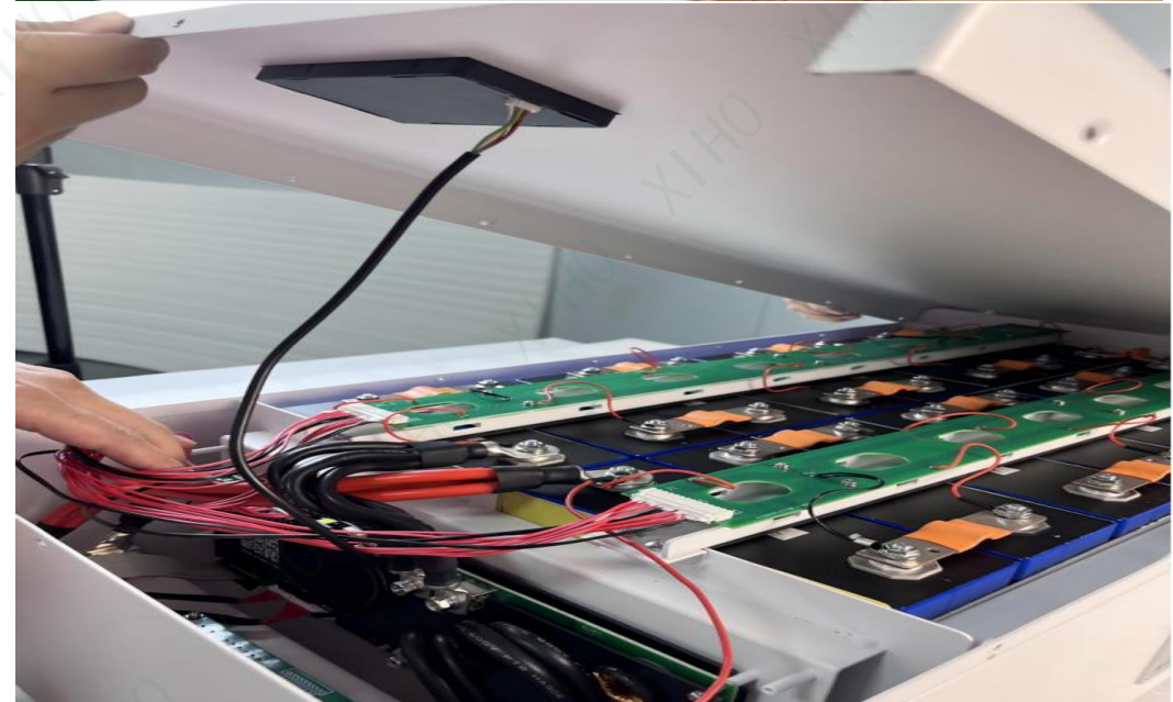
Step12:Install the LED screen onto the cover panel and connect the display cable to the BMS mainboard before closing the cover panel
