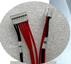
PCB-A Wire Short Wire Line number: #1、#2
