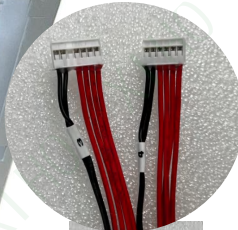
PCB-B Wire Long Wire Line number: #3、#4
