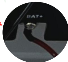
BAT+ Wire (Connect to the Battery Pack Main Positive Terminal)
