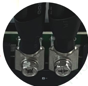
B- Cable (Connect to the Battery Pack Main Negative Terminal)
